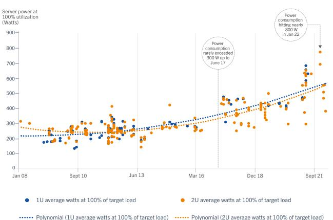
Data is showing sustained maximum power consumption of 2-socket servers when running the SPECpower\_ssj2008, which simulates a Java-based business logic. Results for 1U and 2U form factors. Data as of June 27, 2022.
